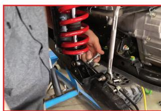
Set "zero Preload" by pressing down on trailing arm and holding to fully extend internal bump stop spring. Rotate preload ring clockwise until spring stack contacts preload ring. This is your "zero preload" point. From here you can set additional preload by tightening the crossover rings. \*Additional Preload may be needed depending on after-market accessories 4-6 turns from zero is a good starting point.
