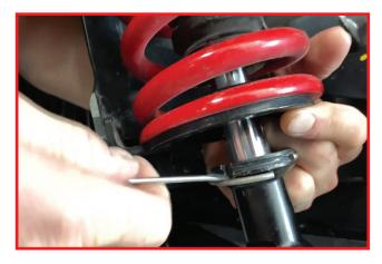
You will NOT need to cut or modify the OEM spring retainer on the front shock kit.
