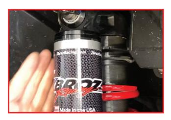
Pull the lower bumpstop up out of the way and push up on the shock guard in order to reveal and remove the spring retainer clip.
