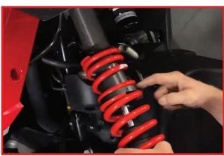
Install new tender spring stack, main spring, lower spring clip.
