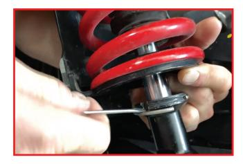
Next, you will need to cut the OEM spring retainer down to 2" Long. Using a measuring device mark 2" down from the bottom of the top spring divider ring.
